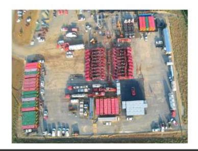
Massive frac-pumping equipment, water tanks, and proppant-sand boxes in place and ready for a new-technology shale-fracking operation.
